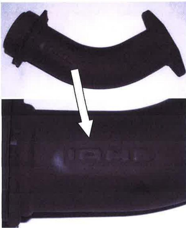
STATOR IDENTIFICATION MARKING
